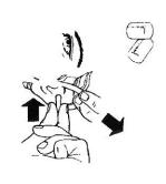
co-worker cannot see the plug while looking straight at you. compressed, insert plug well into the ear canal so you cannot see it head to pull the ear outward and upward during insertion. While Inserting Formable Plugs - Slowly roll and compress foam plugs while looking at yourself while looking straight on in a mirror or a into a very thin cylinder. Fitting is easier if you reach around the
